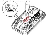
**STEP 4** – Insert required Lens followed by Bezel and re-insert coloured screws and Lid
