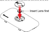
Note: for Corridor Lens ensure the two pins engage into the PCA
